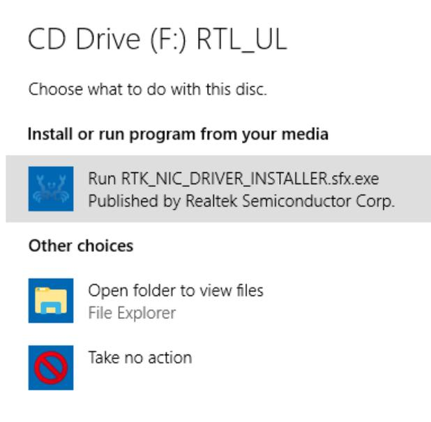
2. The driver will then be installed automatically. Opens up Computer Management, click “System Tools”, “Device Manager”, then “Network adapters”, “Realtek Gaming USB 2.5GbE Family Controller” should appear if the driver is installed successfully.
