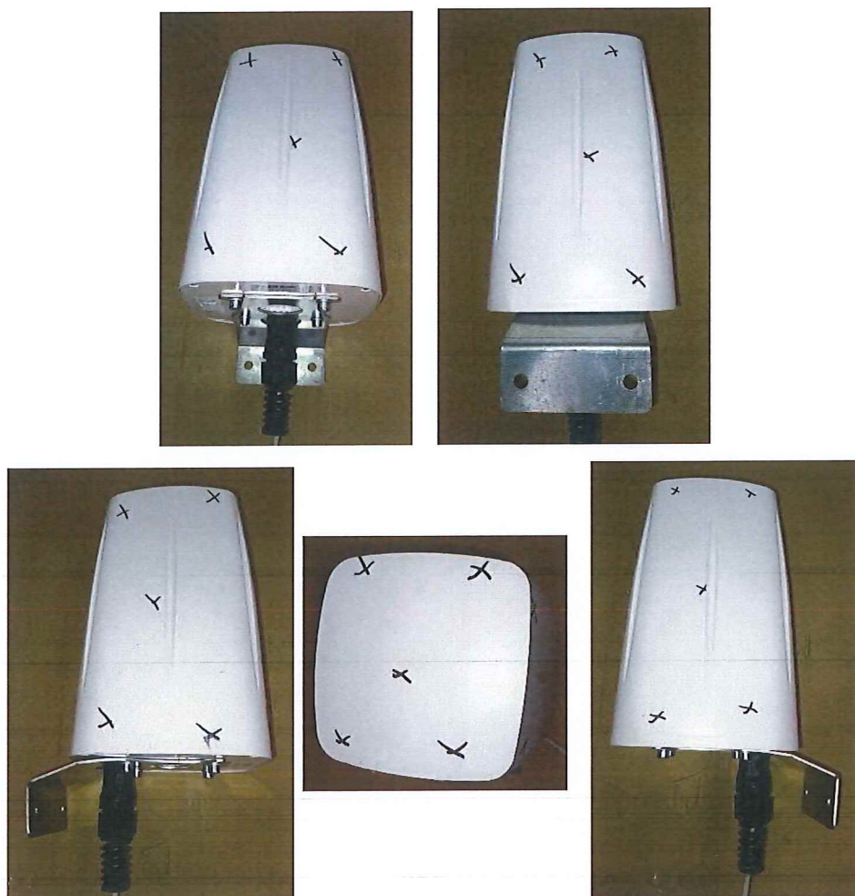
Fig. 4. Points on the surfaces of the enclosure no. 166/24/2 after exposure to mechanical impacts IK08
