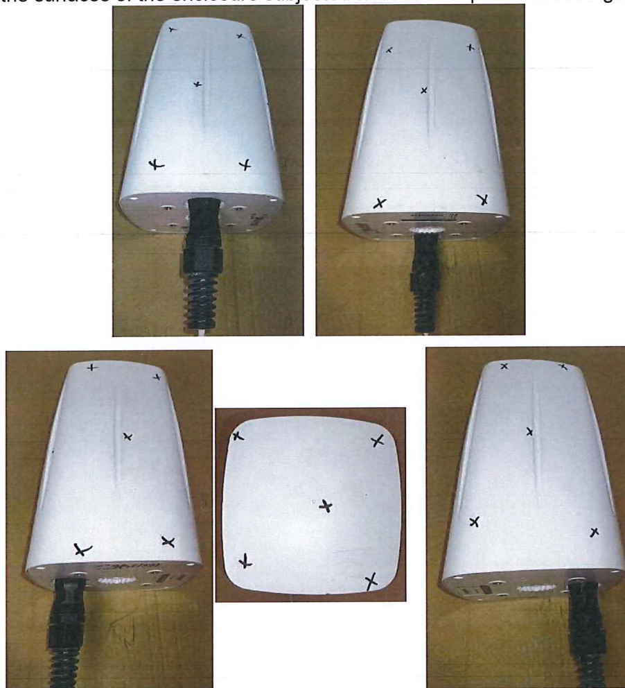
Fig. 3. Points on the surfaces of the enclosure no. 166/24/1 after exposure to mechanical impacts IK08
