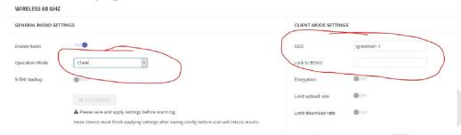
Check the SSID is the same as the Master. Also notice that you can enter the BSSID of the master if you want. This is the MAC address of the 60GHz interface and can be found on the Device Information page for the Master unit
