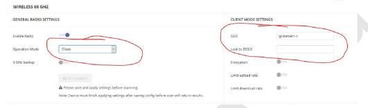
Also you might want to consider adding some encryption of the link data. That is also set in the General Radio Settings for each unit; obviously you have to set encryption on both Master and Clients to the same:
