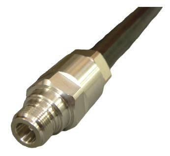
Now screw the front part of the connector onto the back part until hand tight, then tighten the back part of the connector using the two 23mm spanners until it is not possible to tighten anymore
