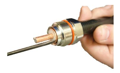
Now use the small flat head screwdriver to flair the copper outer as shown.
