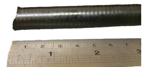
Cut the end of the cable square and clean using a hacksaw, remove all burs and copper dust from the cutting and measure 13mm from the end.
