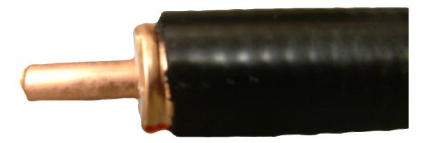
Carefully cut 9mm from the end leaving the solid core centre instact. This is done by using a Stanley knife to cut straight through the copper outer and the white ptfe insulator down to the solid core.
