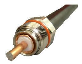
Push the back part of the connector onto the cable, it should pass over the black jacket and leave the remaining copper jacket just poking out.
